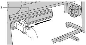
4 Insert the media core onto the center hubs of the take-up holders.
